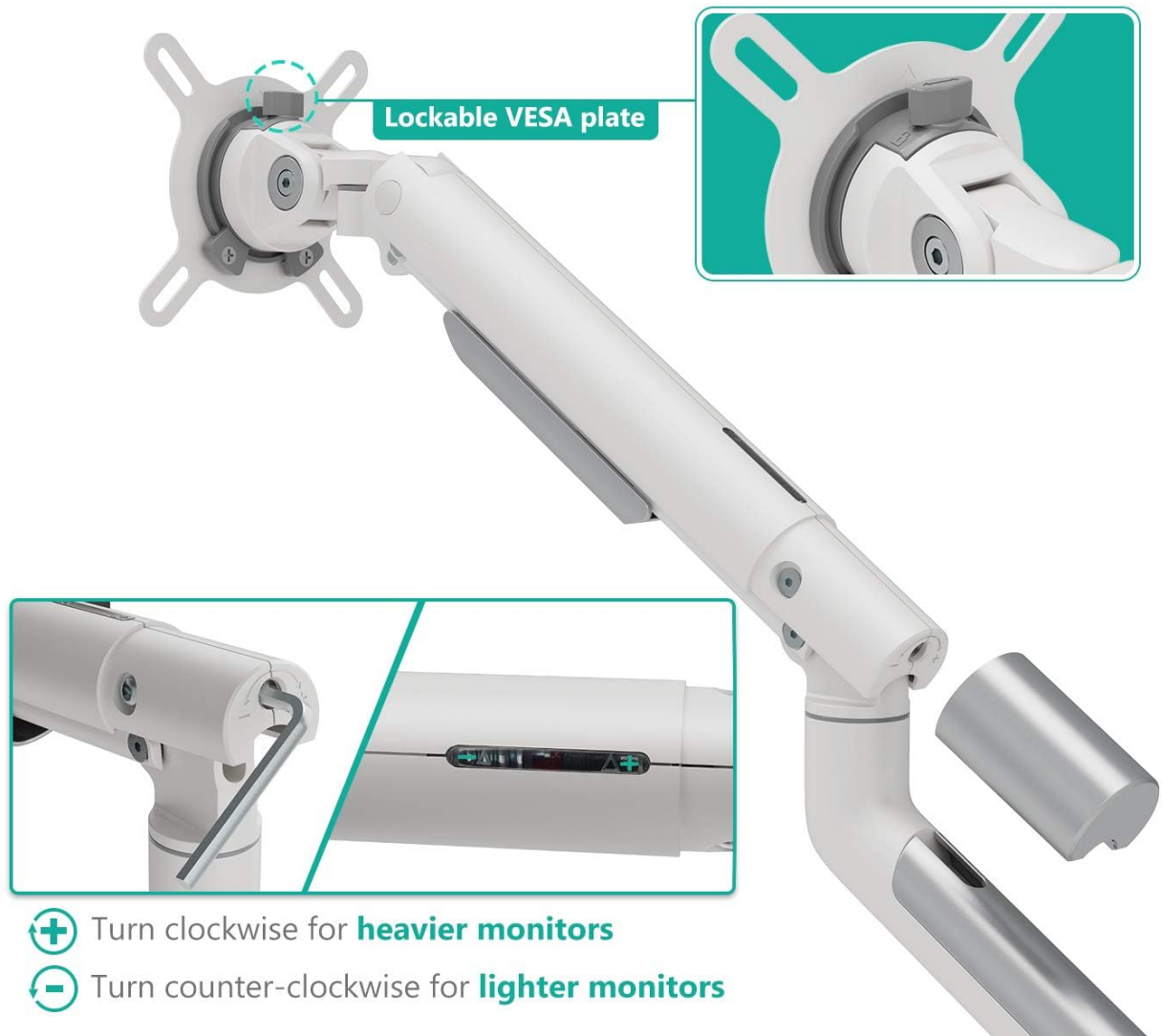
Figure 3: Built-in Tension Indicator. This image highlights the lockable VESA plate and the built-in tension indicator on the monitor arm. The indicator helps in aligning multiple monitors and adjusting the spring tension. Turning clockwise increases tension for heavier monitors, while turning counter-clockwise decreases tension for lighter monitors.
