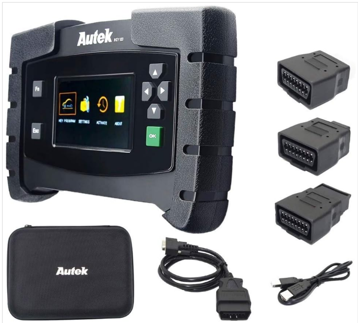
Figure 2.2: Detailed view of the IKEY820 Pro device highlighting key buttons and ports. These include the Fn Key, Main Cable Port, ESC Key, USB Port, Power Port, OK Key, and directional navigation keys.
