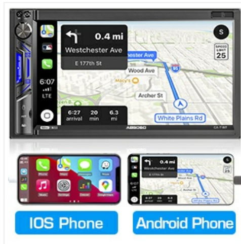
Image 5.4: The Phone Link feature mirroring a smartphone's navigation app onto the car stereo screen.
