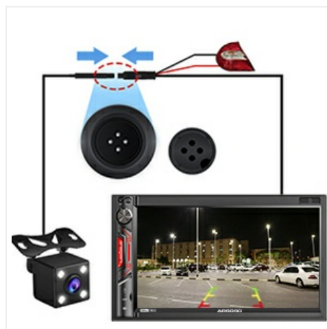
Image 4.2: Illustration of connecting the backup camera to the car stereo system.
