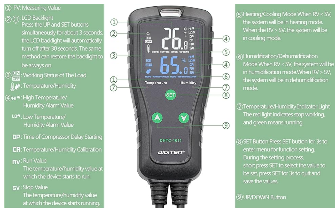
Figure 2.3: Detailed view of the controller's display and buttons. (1) PV: Measuring Value, (2) LCD Backlight, (3) Working Status of the Load (ON/OFF), (4) High/Low Temperature/Humidity Alarm Value (HI/LO), (5) Heating/Cooling Mode (RV < SV: Heating, RV > SV: Cooling), (6) Humidification/Dehumidification Mode (RV < SV: Humidification, RV > SV: Dehumidification), (7) Temperature/Humidity Indicator Light (Red: Stop, Green: Running), (8) SET Button, (9) UP/DOWN Button. DP: Time of Compressor Delay Starting, CA: Temperature/Humidity Calibration, RV: Run Value, SV: Stop Value.
