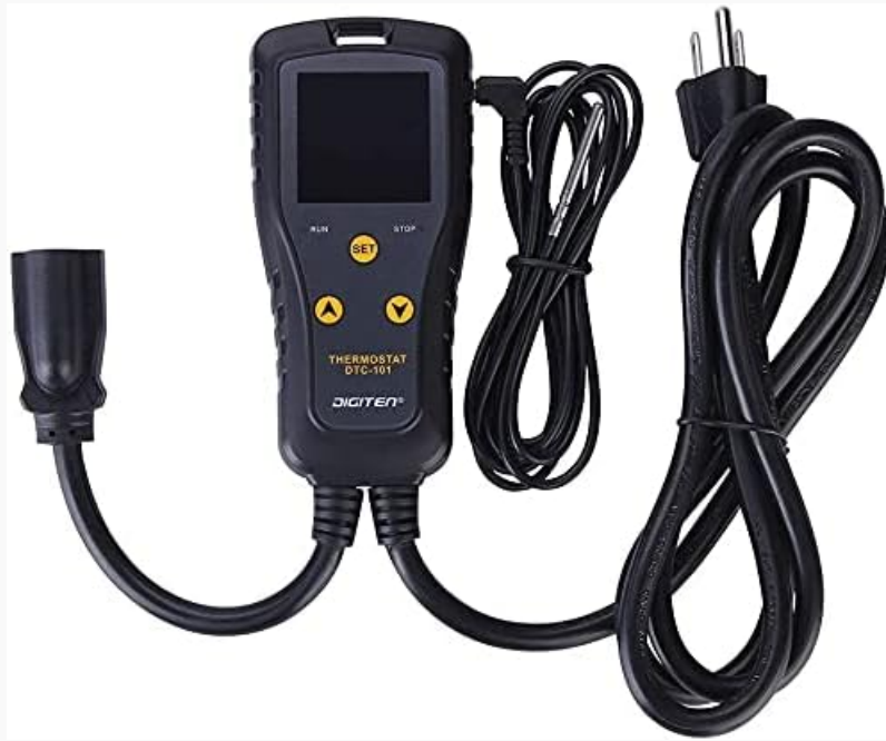
Figure 2: Controller unit with power and output cables
