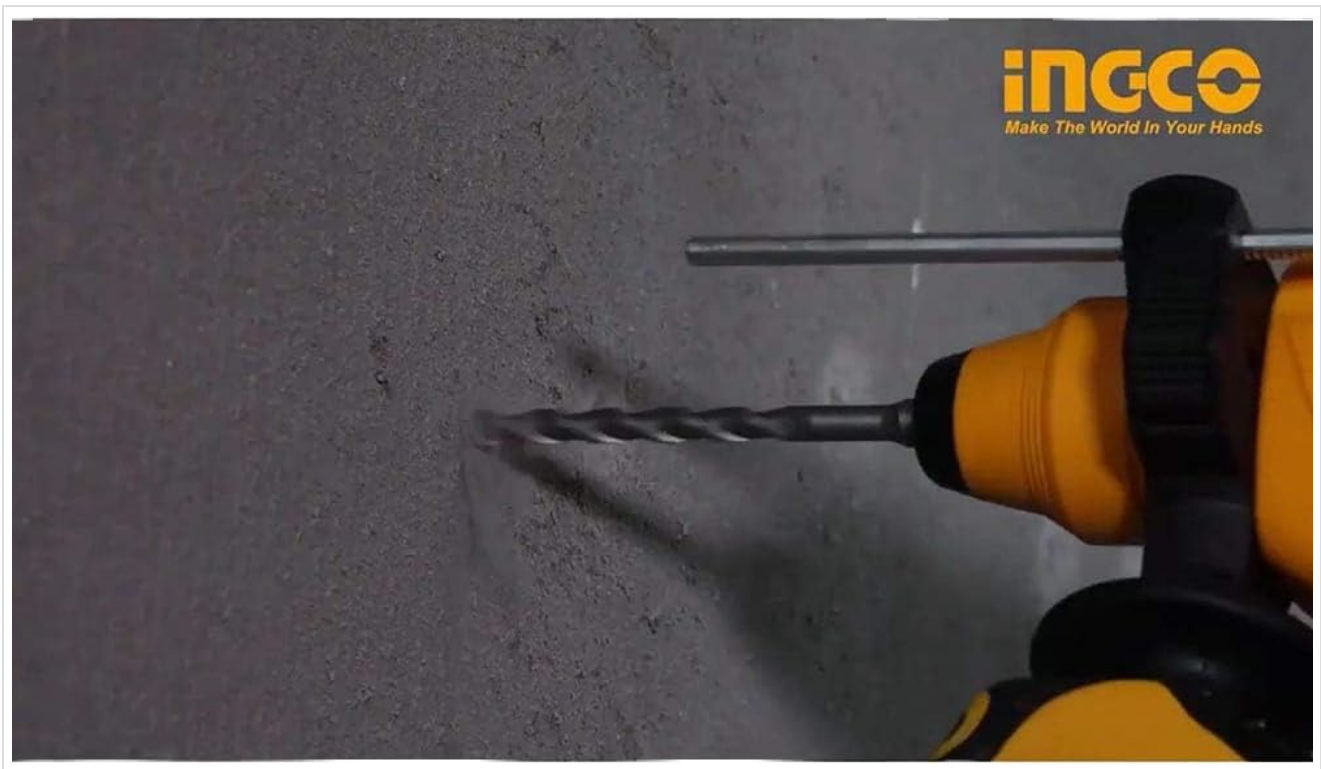
Figure 5.1: The Ingco RGH9028 Rotary Hammer Drill being used for drilling into a concrete surface, demonstrating proper grip and application.
