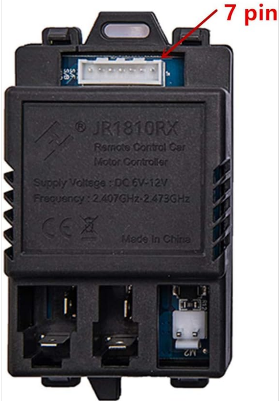
A detailed view of the JR1810RX control box highlighting the 7-pin connector, essential for proper installation in children's electric cars.
