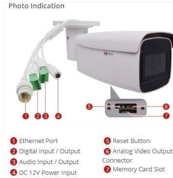
Figure 3.1: Photo Indication of the ACTI CORPORATION A418 camera's ports and connections. This diagram labels the Ethernet Port (1), Digital Input/Output (2), Audio Input/Output (3), DC 12V Power Input (4), Reset Button (5), Analog Video Output Connector (6), and Memory Card Slot (7).
