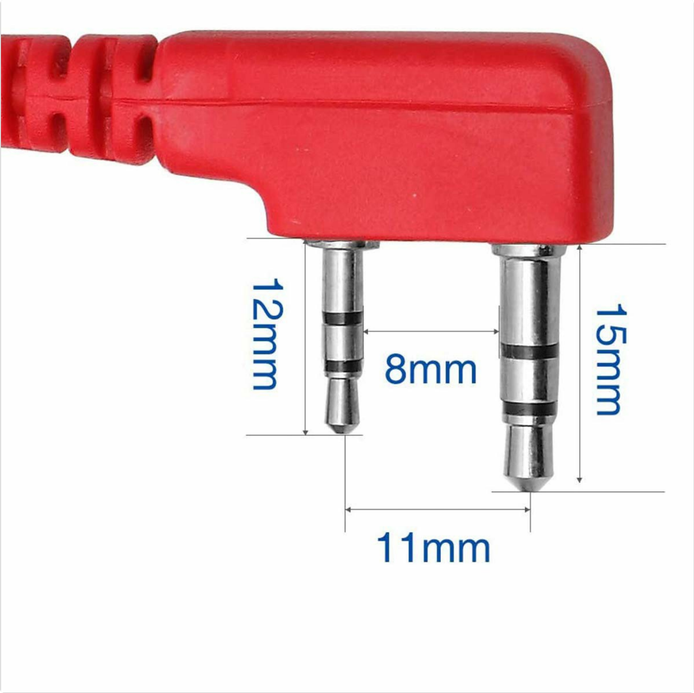
Figure 4: Detailed measurements of the two-pin K-type connector, showing pin lengths of 12mm and 15mm, and an 8mm spacing between them, with an 11mm width.
