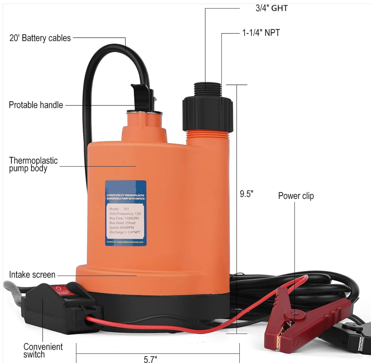
Image: Side view of the FLOWPAC FX701-Orange submersible pump, highlighting its thermoplastic pump body, portable handle, intake screen, convenient switch, 20' battery cables, 1-1/4" NPT discharge, 3/4" GHT adapter, and power clips. Dimensions of 9.5" height and 5.7" width are indicated.
