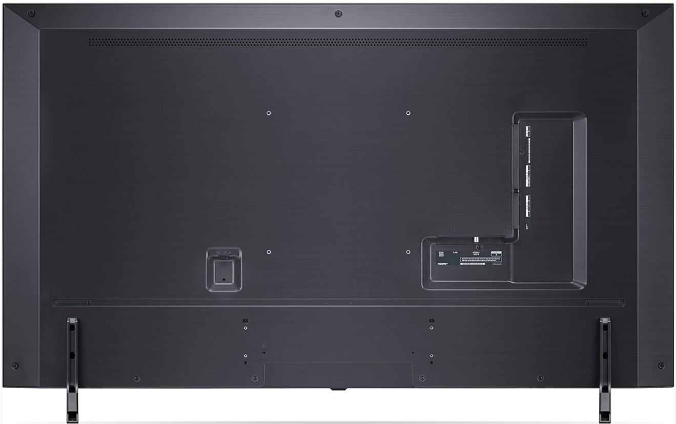
Rear view of the TV highlighting the various input ports for external devices.
