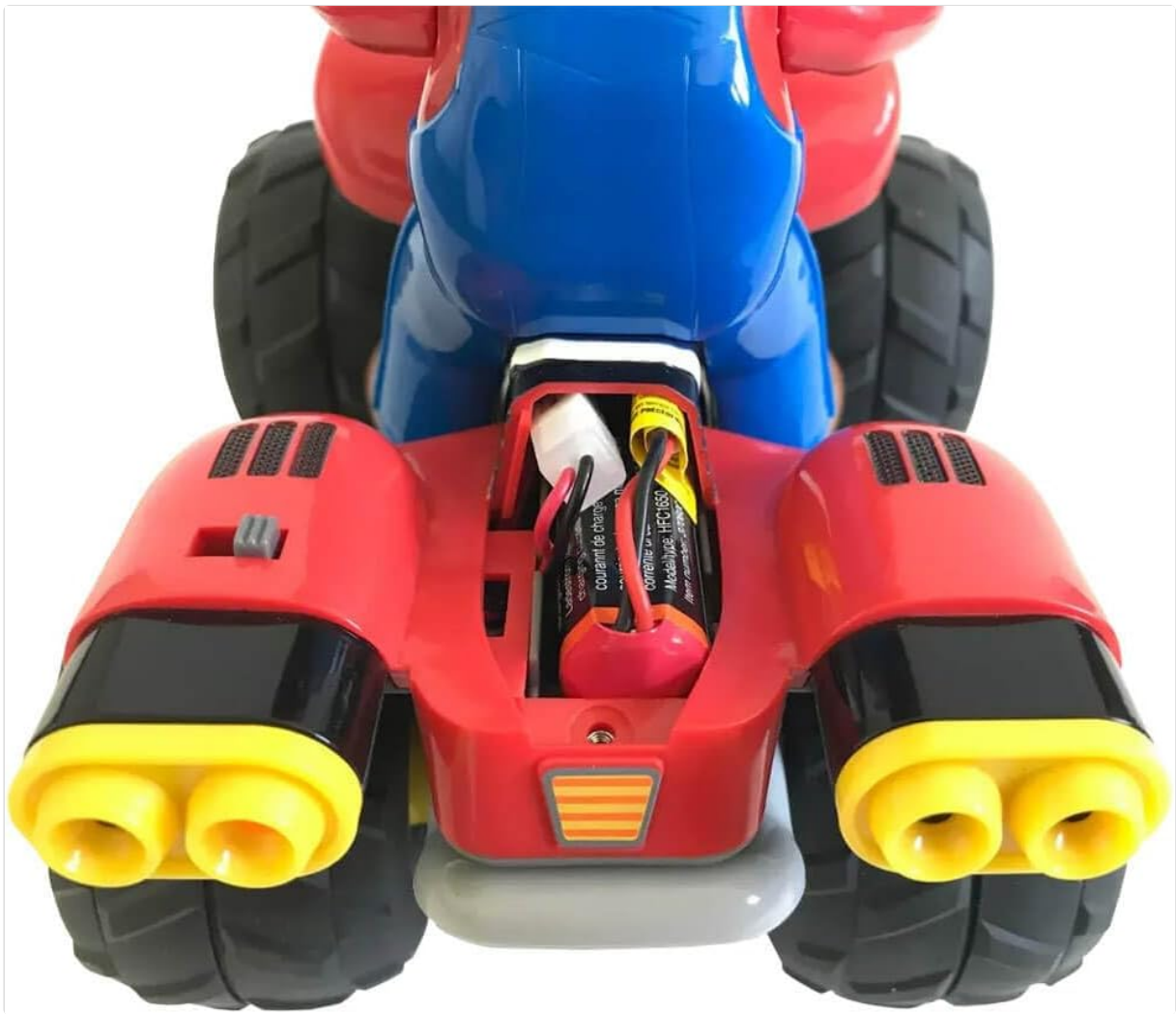
Image 2: Battery compartment of the Mario Kart Quad. This image shows the location and method for installing the rechargeable LiFePO4 battery in the vehicle.
