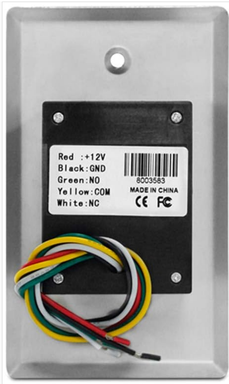
Figure 5.1: Rear view of the LBS Touchless Exit Button Switch showing the wiring terminals. Labels indicate Red: +12V, Black: GND, Green: NO, Yellow: COM, White: NC.
