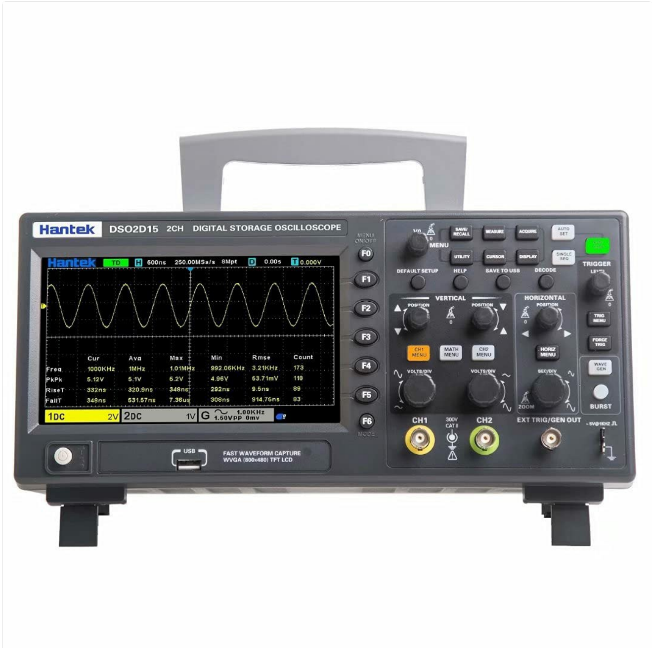
Figure 4.1: Front panel of the DSO2D15, showing the display, function buttons (F1-F6), vertical and horizontal controls, trigger controls, and channel inputs.
