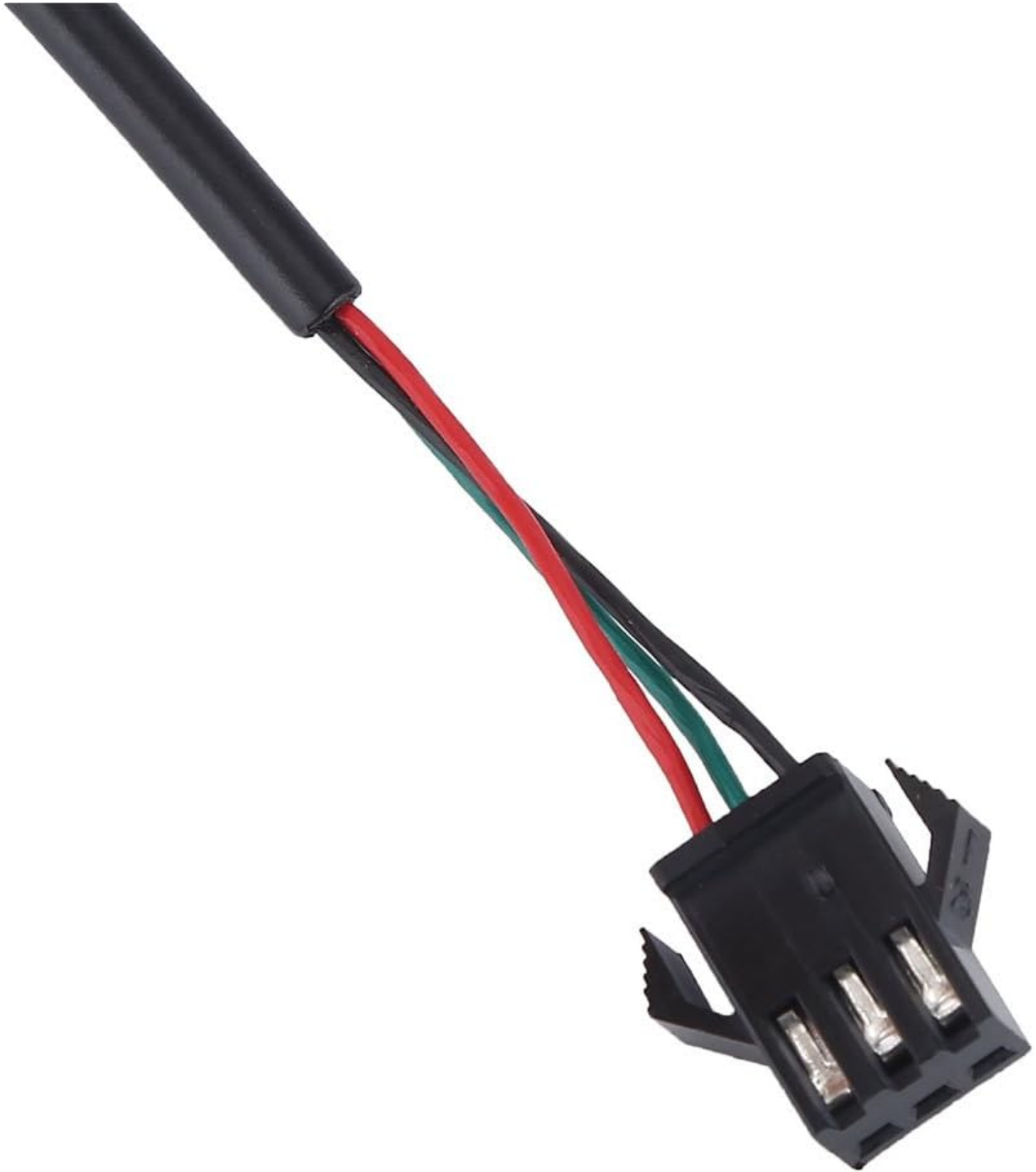
Image 2.2: Detailed view of the 3-wire connector, showing the black, green, and red wires.
