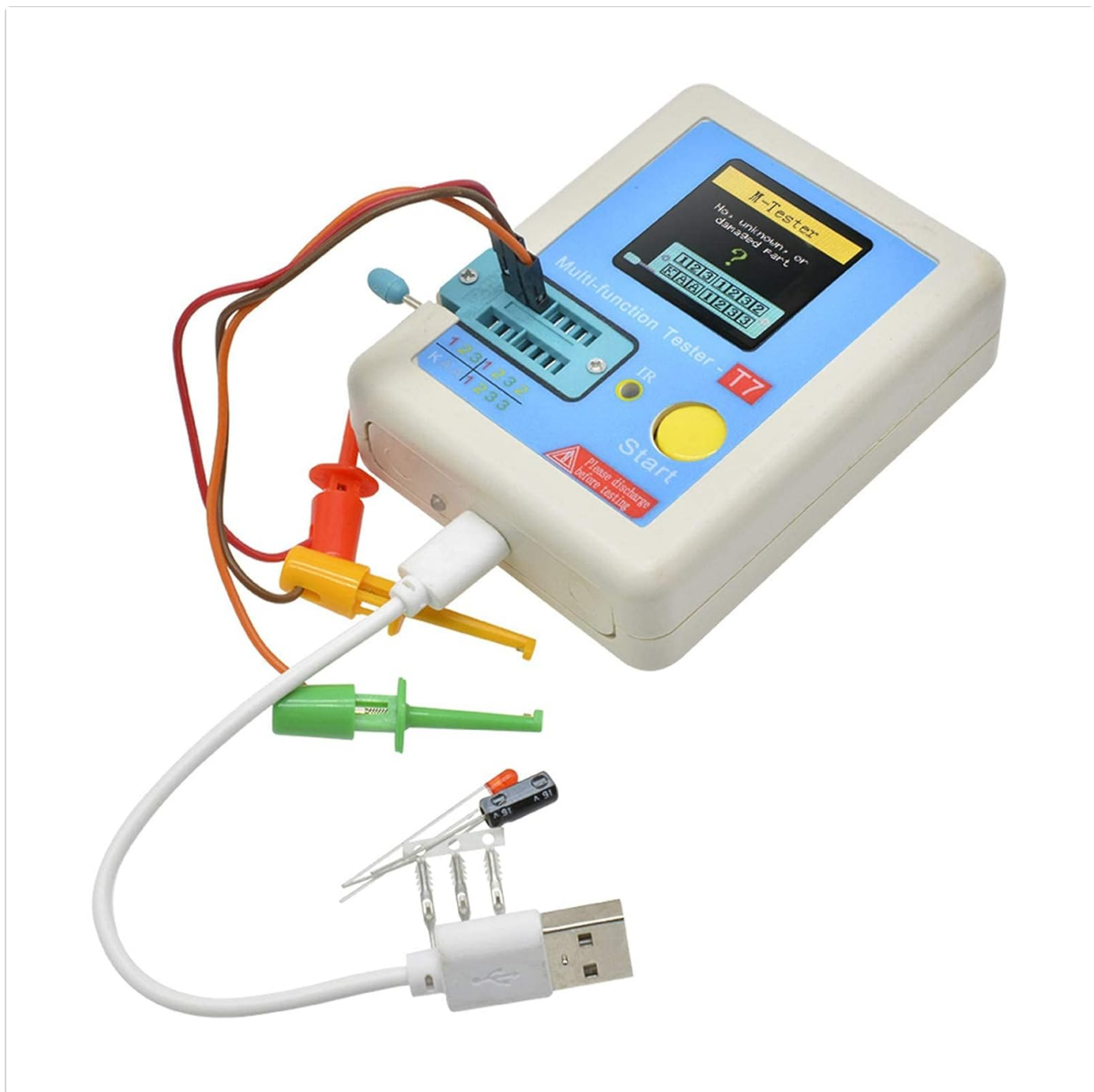
Figure 4: The LCR-T7 tester connected to a component using test clips for measurement.
