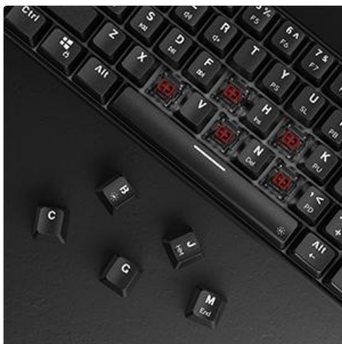
Image: Demonstration of how to remove keycaps from the keyboard, a necessary step before accessing switches.
