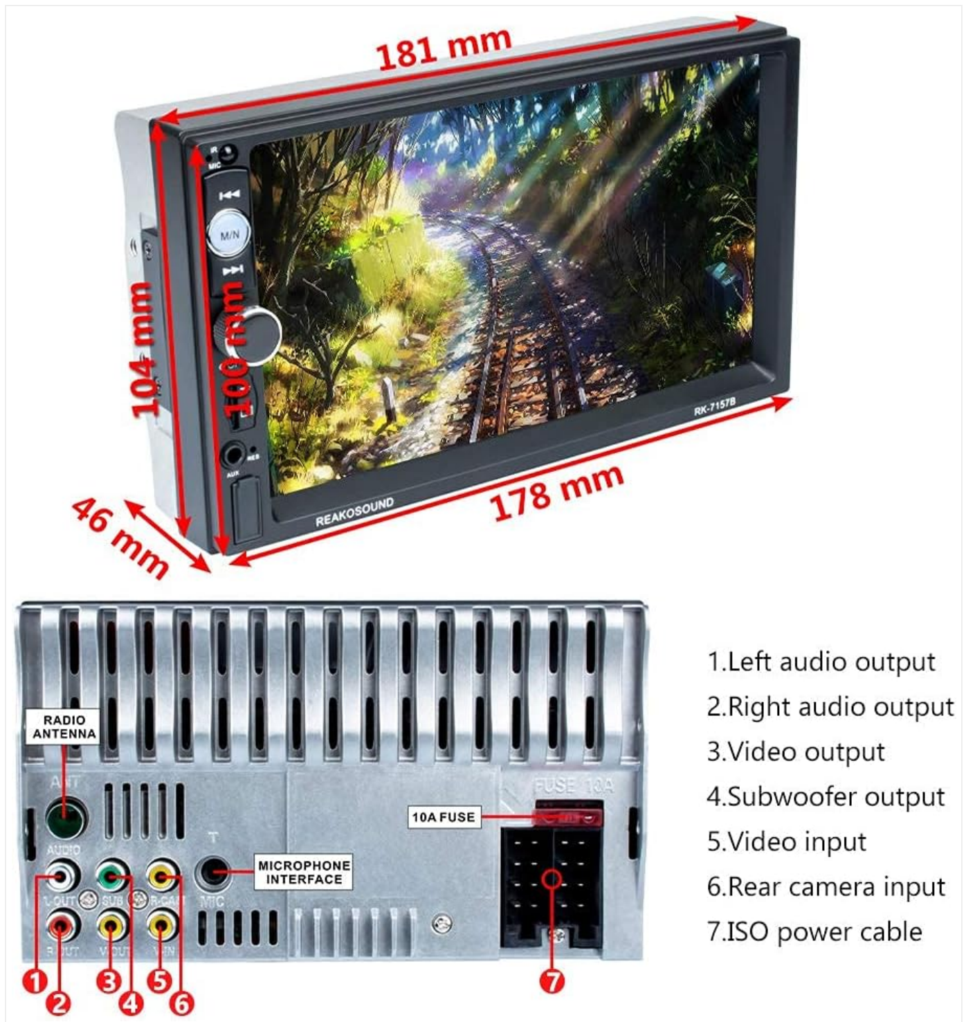
Figure 4.1: Rear connections and dimensions of the car stereo.
