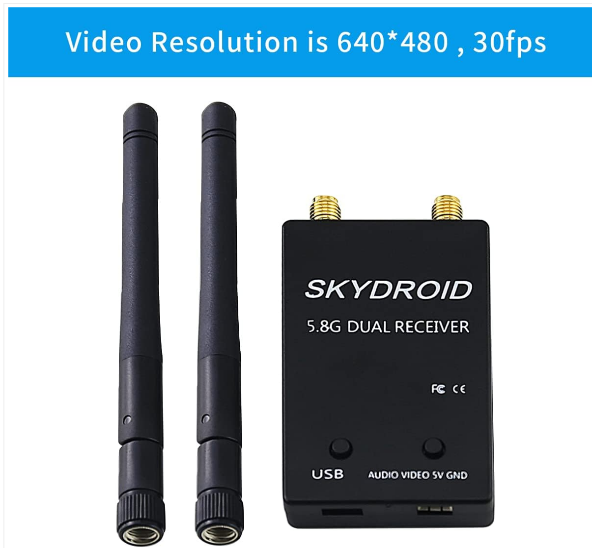
Image: The FPV receiver supports a video resolution of 640x480 pixels at 30 frames per second.
