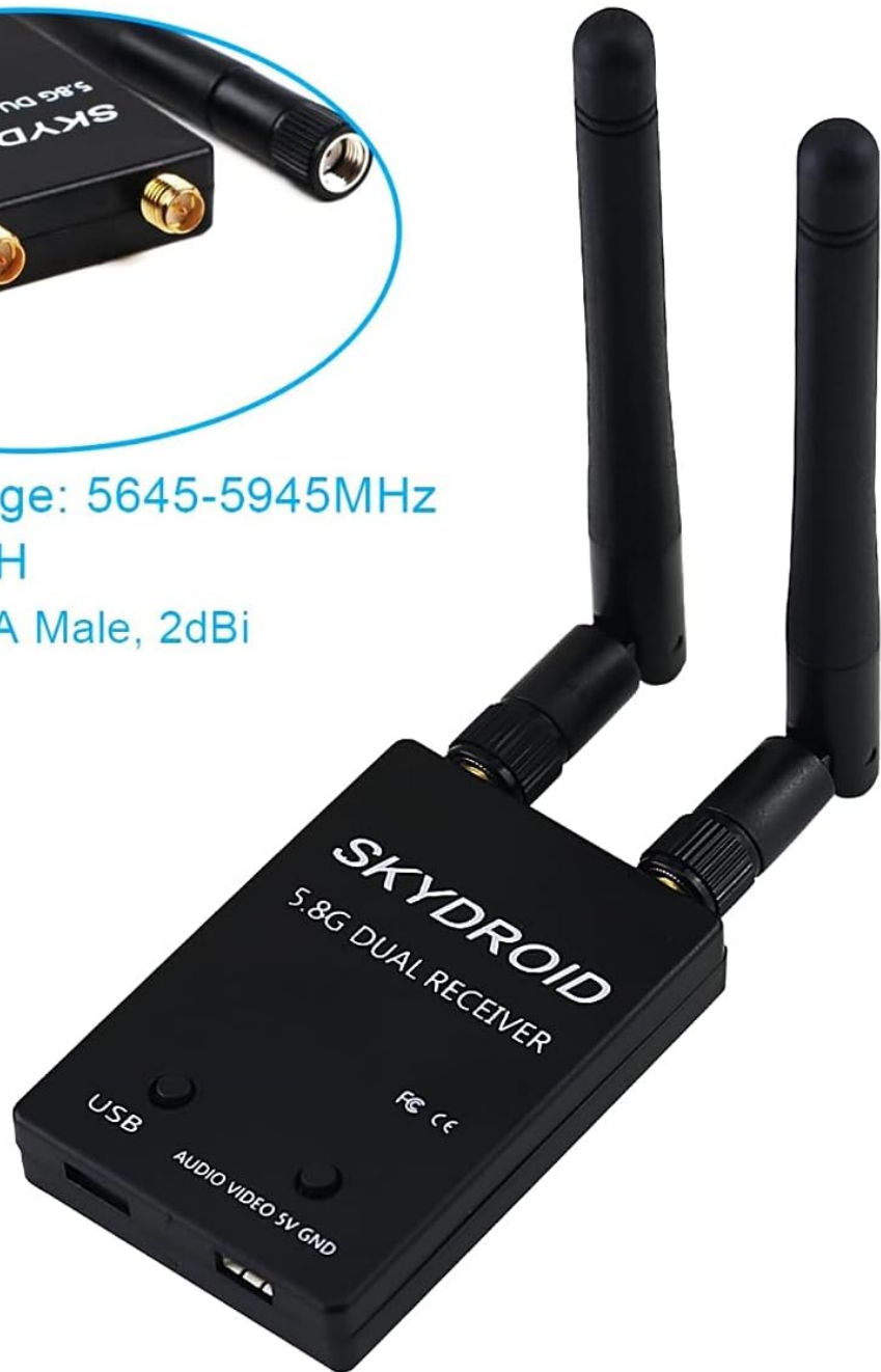
Image: Front view of the SKYDROID 5.8G Dual Receiver, highlighting its frequency range (5645-5945MHz) and 150 channels. It features two RP-SMA Male, 2dBi antennas.
