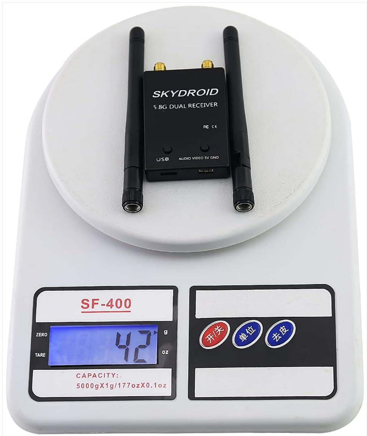
Image: The FPV receiver weighs approximately 42 grams (1.48 ounces).
