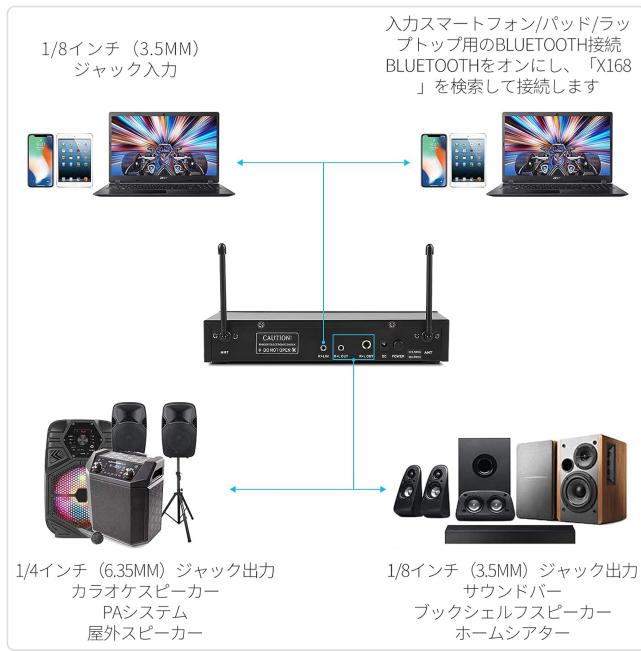
This diagram provides a comprehensive overview of the input and output connections available on the XTUGA UH330 receiver. It shows how to connect the system to various audio devices like smartphones, laptops, karaoke speakers, PA systems, soundbars, and home theater systems using different cable types (3.5mm, 6.35mm, RCA).
