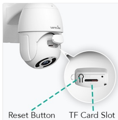
Figure 2: Reset Button and TF Card Slot Location.
