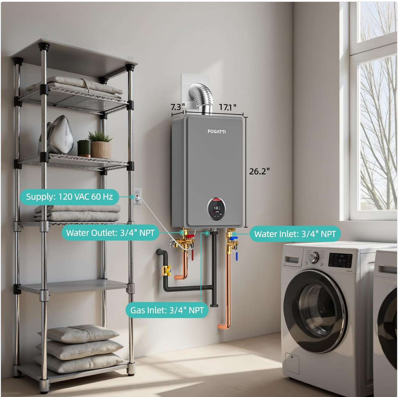
Installation Diagram: The unit measures 26.2"H x 17.1"W x 7.3"D. It requires a 120 VAC 60 Hz supply. Water Inlet and Outlet are 3/4" NPT, and Gas Inlet is also 3/4" NPT.
