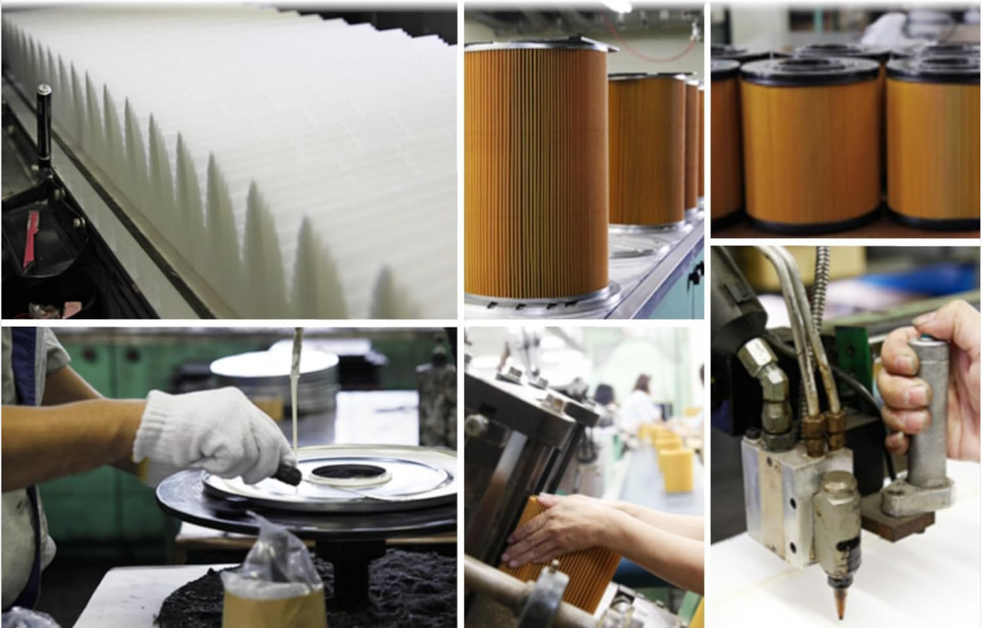
Figure 3: The ALPS AA-7762 air filter element, showing its pleated design for maximum filtration surface area.
