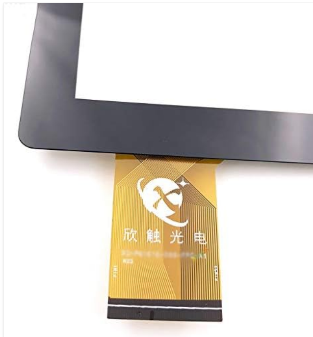
Image: A close-up view of the digitizer's flex cable, which connects to the tablet's main board.
