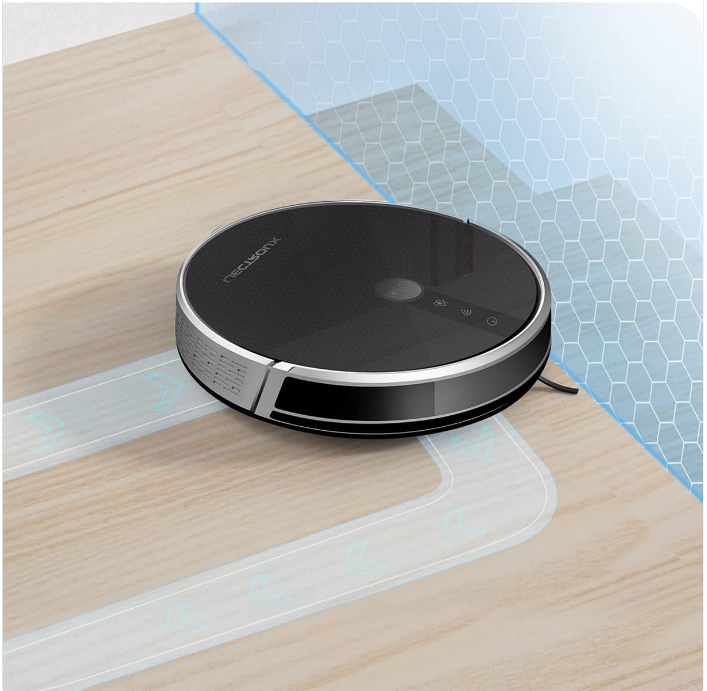
Figure 7.1: The robot is equipped with anti-drop sensors that detect changes in elevation, such as stairs, preventing it from falling and ensuring safe operation.
