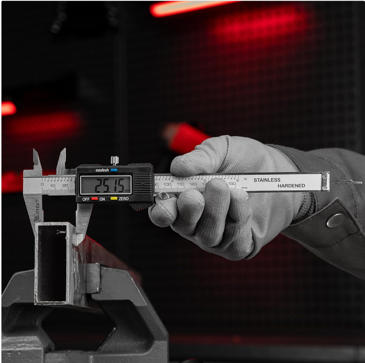
Figure 4: Measuring an external dimension.
