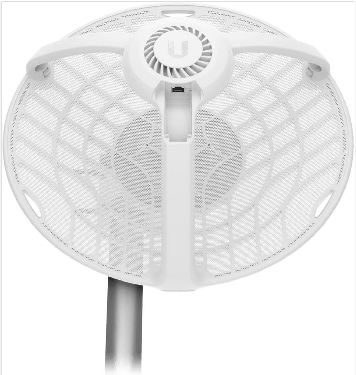
Figure 4: Rear view of the AF60 LR with the protective cover removed, revealing the Ethernet port and the reset button for device management.
