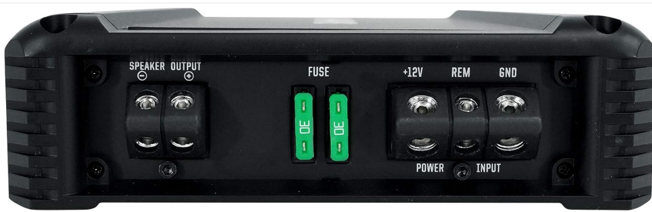
Figure 4.2: Amplifier power and speaker output terminals.
