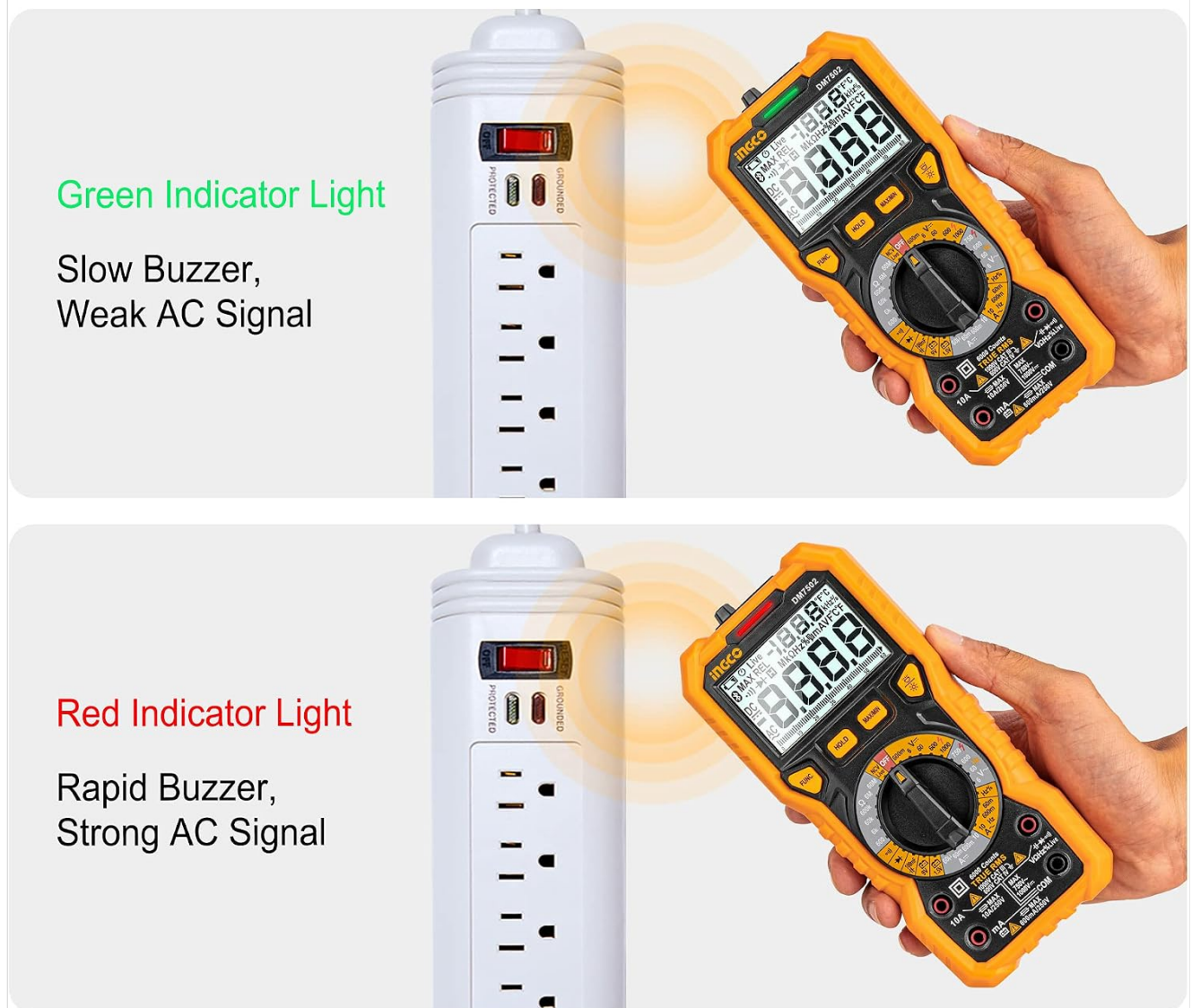
Figure 5.3: Illustration of the NCV function, showing how the multimeter detects AC signals and indicates strength with different colored lights.
