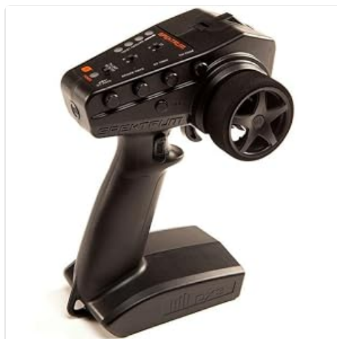
Figure 4: The Spektrum DX3 3-Channel 2.4GHz DSMR Radio Transmitter, used for controlling the vehicle.
