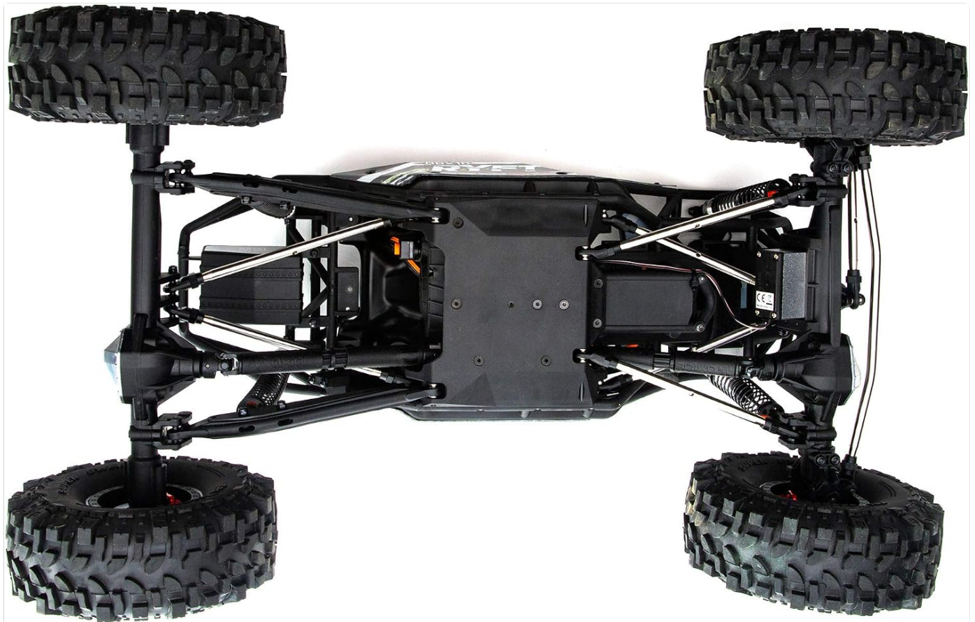
Figure 3: Top view of the Axial RBX10 Ryft chassis, showing the battery secured within its compartment.
