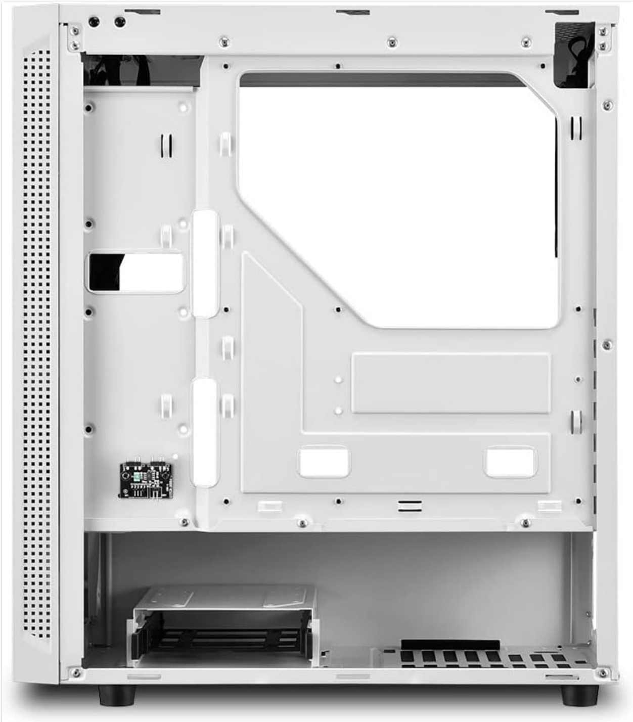
Image 4.2: Rear interior view, highlighting cable management options and locations for 2.5" SSDs and 3.5" HDD cage.
