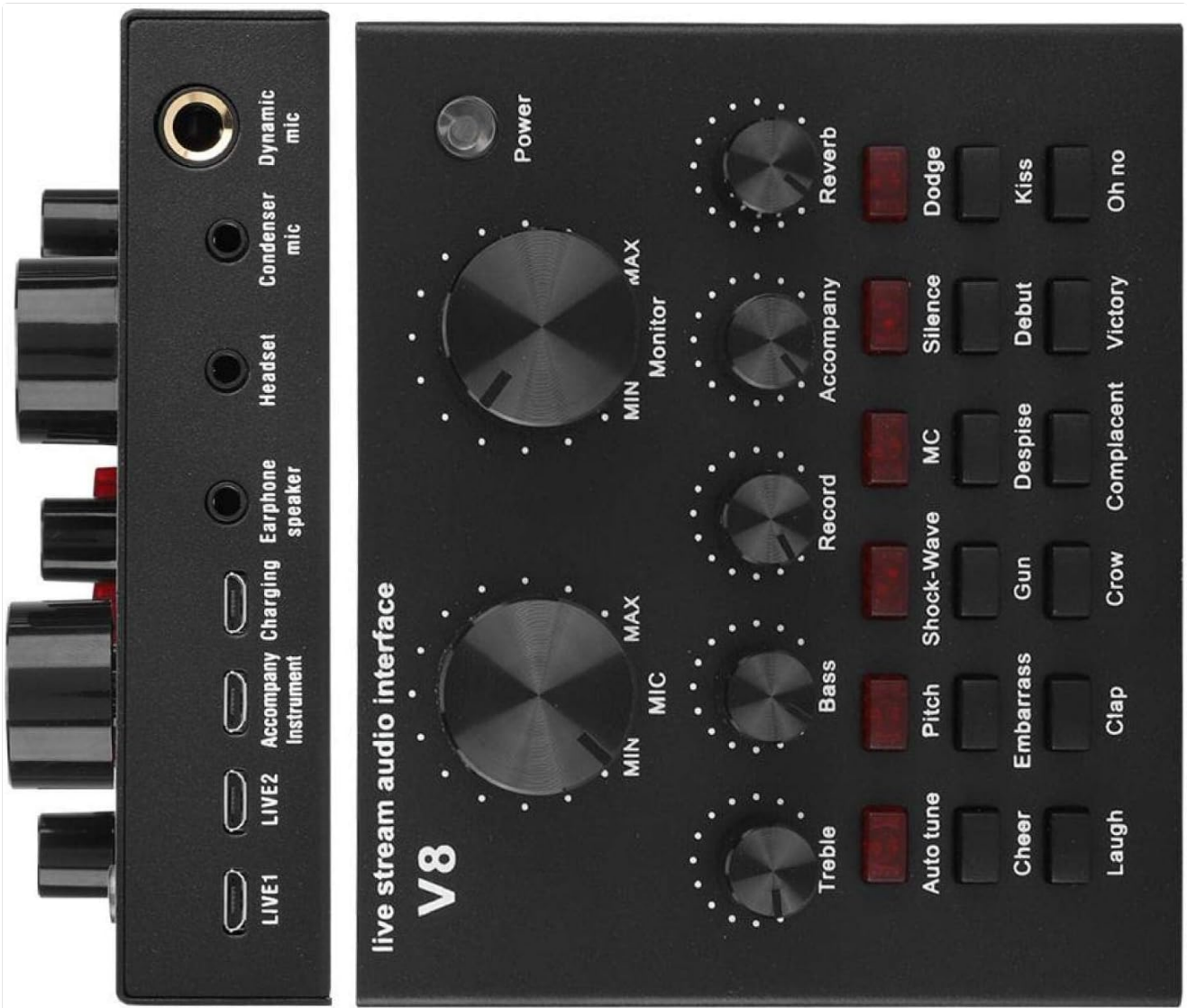
Side view illustrating the various input and output ports for microphones, headsets, and live connections.
