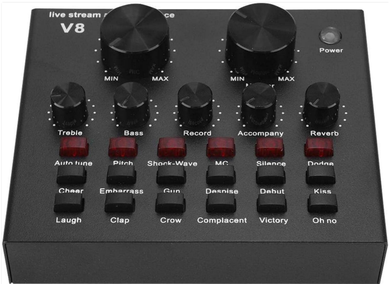
Detailed view of the sound card's control panel, showing knobs and effect buttons.
