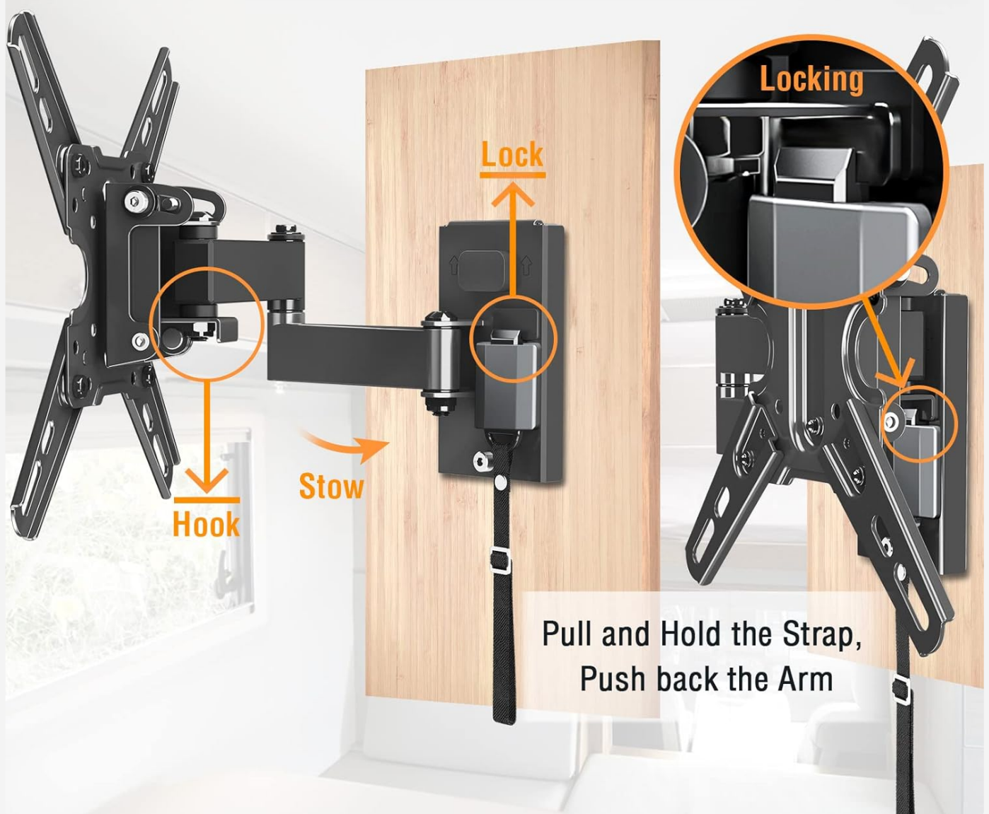
Image 5.2: Engaging and disengaging the one-step locking mechanism.
