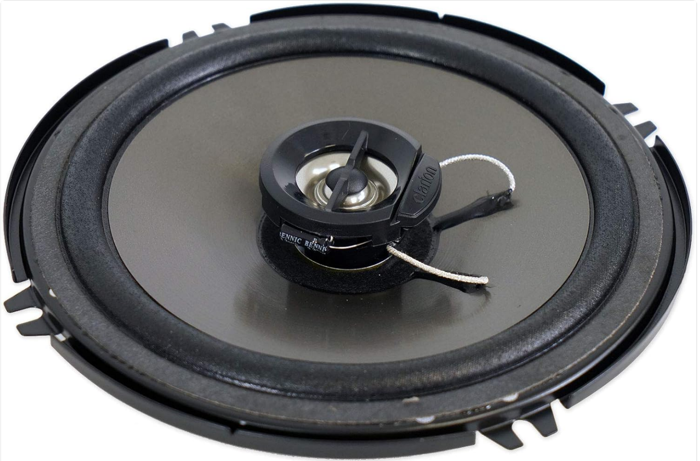
Figure 4.1: Detail of the MIPP cone and tweeter.
