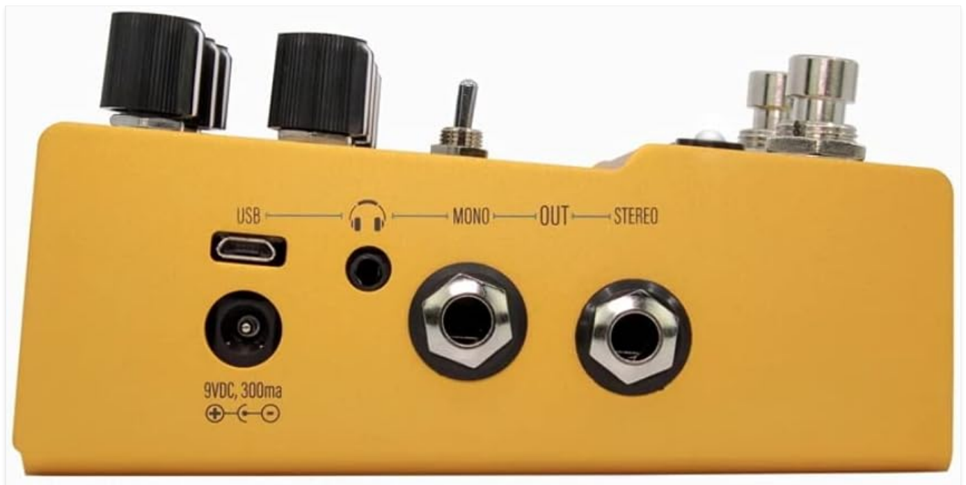
Figure 2: Rear view of the ACS1 showing the 9VDC power input, USB port, headphone jack, and mono/stereo outputs.
