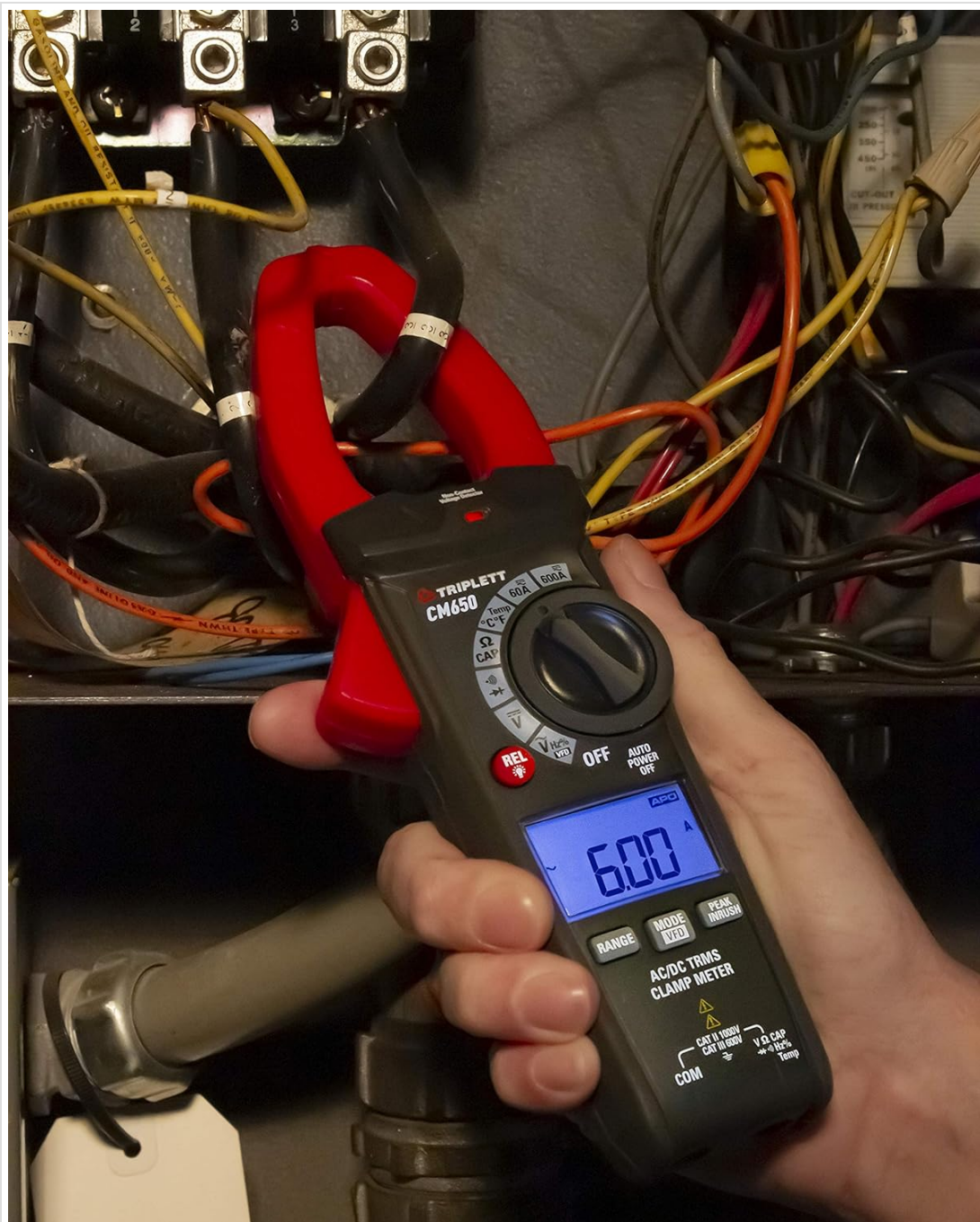
Figure 4.1: A hand holding the Triplet CM650 clamp meter, with its jaws clamped around a single wire within an electrical panel, demonstrating how to measure current. The display shows a reading of 60.0 A.
