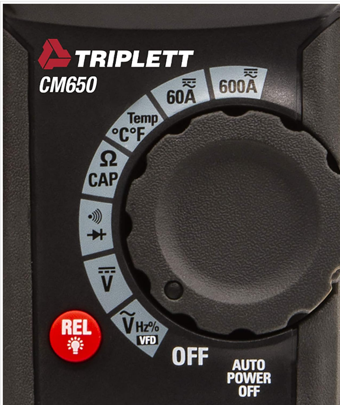
Figure 2.2: Close-up view of the Triplet CM650's rotary dial and function buttons. This image highlights the various measurement selections such as 60A, 600A, Temperature, Resistance/Capacitance, Continuity/Diode, Voltage, and VFD mode, along with the REL and backlight button.
