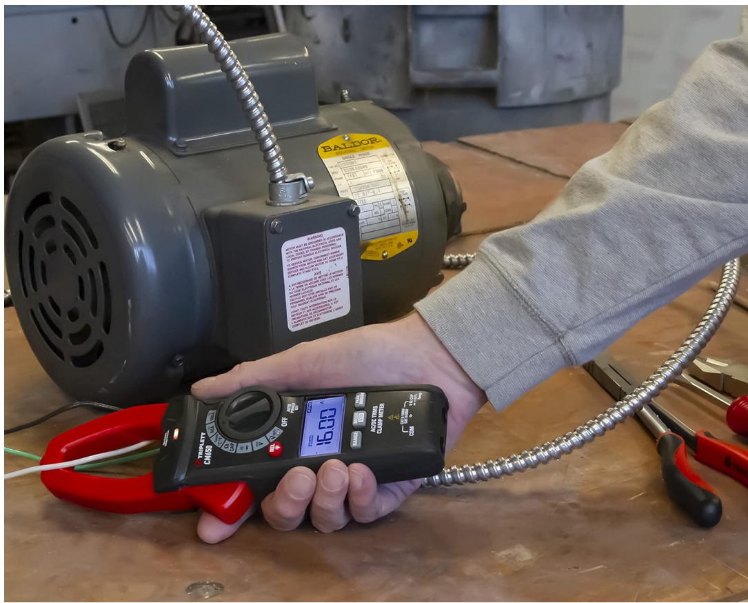
Figure 4.2: The Tripplett CM650 clamp meter being used to measure current on a wire connected to an industrial motor. The meter's display shows a reading of 16.00 A, illustrating its application in industrial settings.
