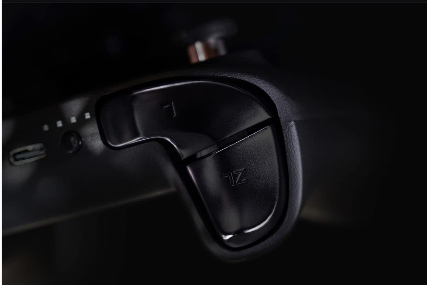
Figure 7: Hall sensing ZR, ZL analog triggers offer high accuracy, contactless operation, and long life.
