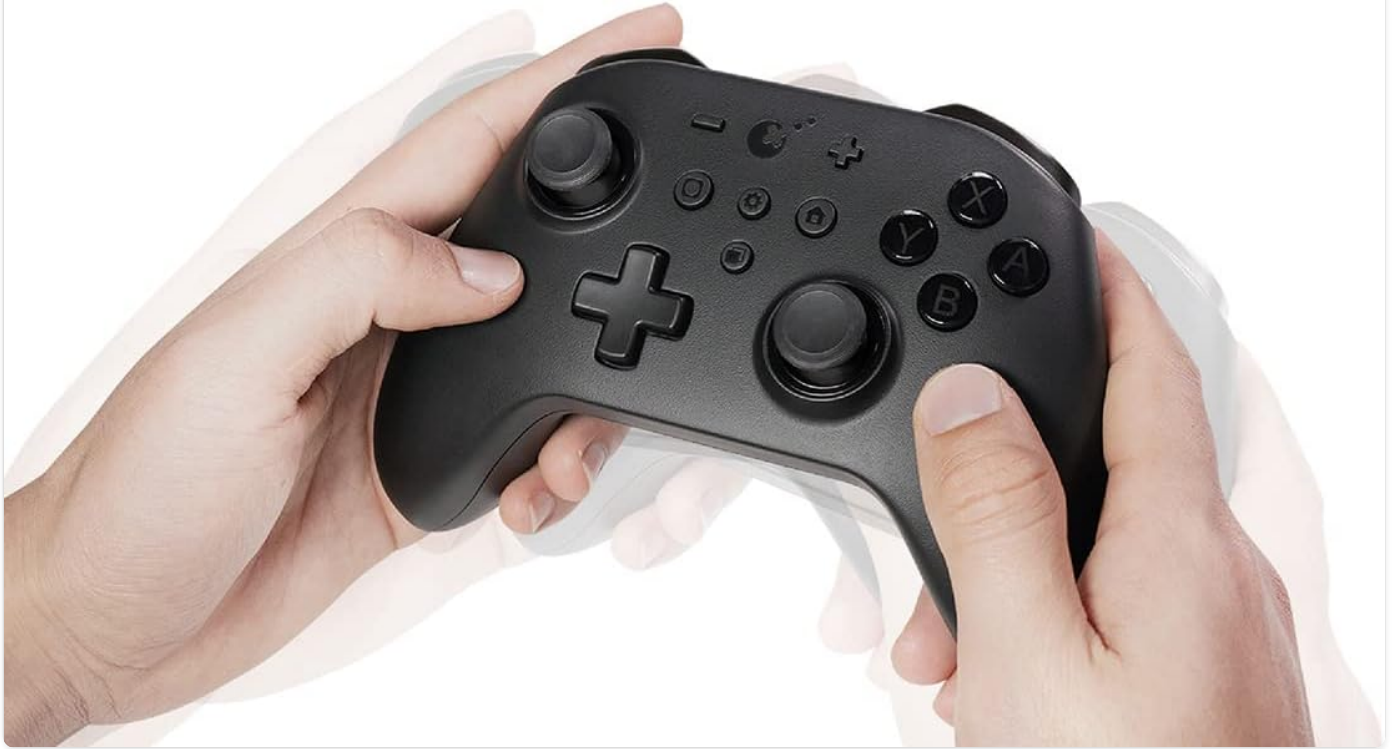
Figure 9: The controller features a built-in acceleration sensor and six-axis gyroscope to support motion sensing on Switch.
