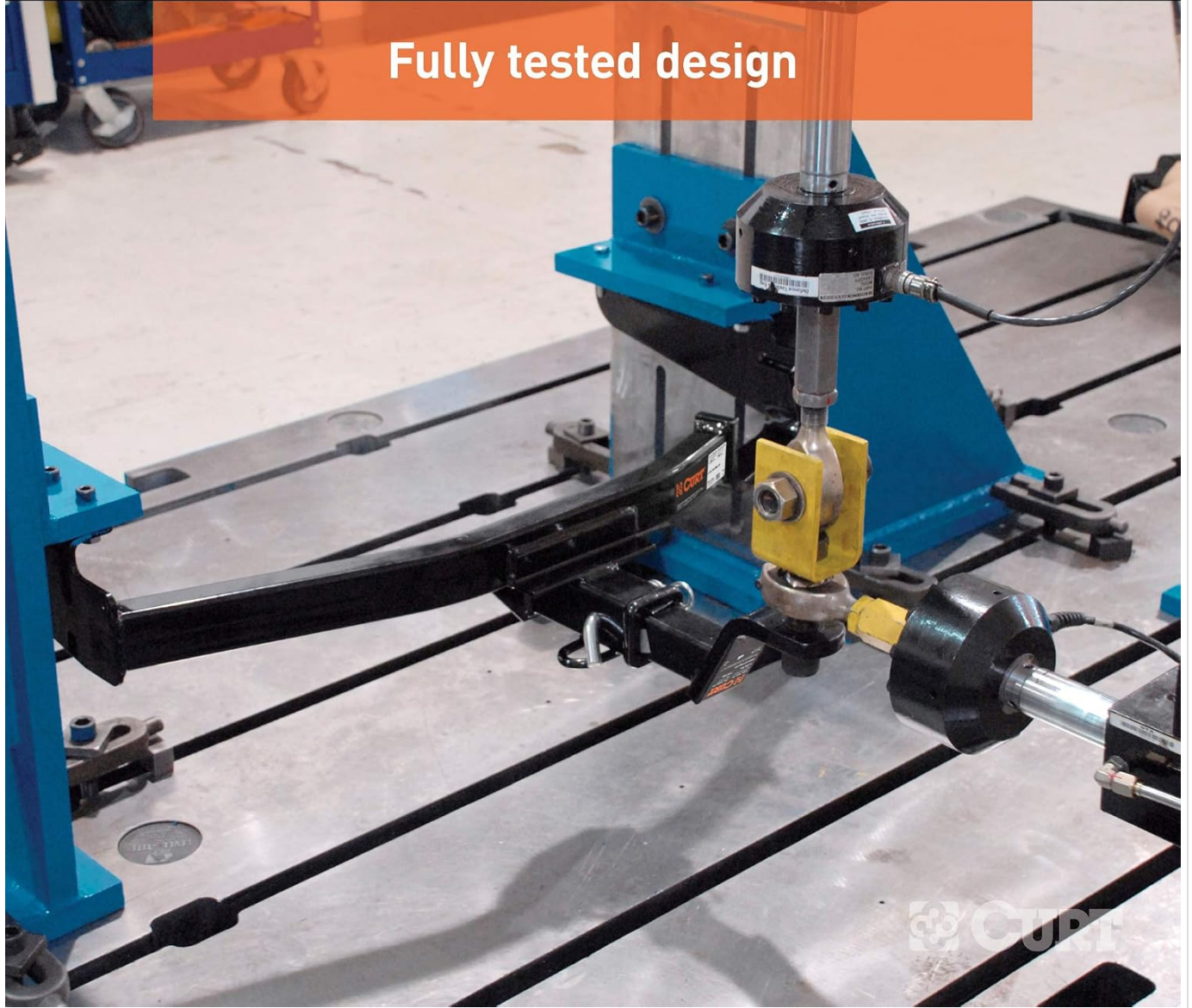
Image 2.5: A CURT hitch undergoing rigorous testing to ensure it meets safety and performance standards.
