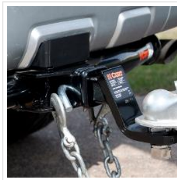
Image 6.2: A close-up view of a hitch connection, showing the ball mount, hitch pin, and properly crossed safety chains.
