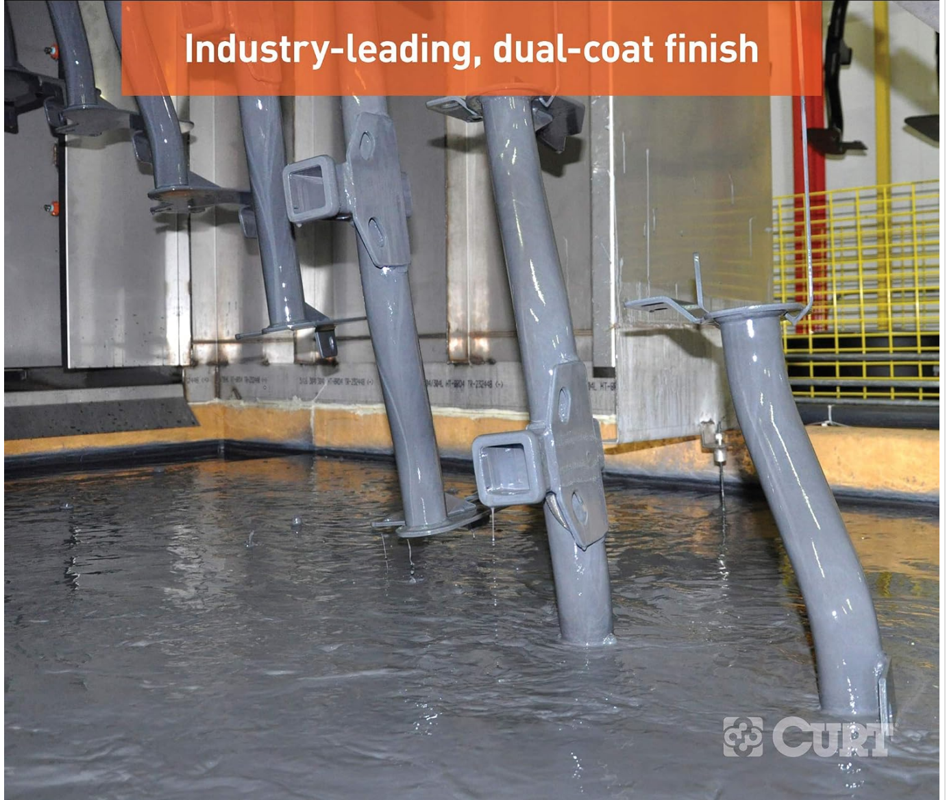
Image 2.4: Components undergoing the dual-coat finishing process, which provides enhanced durability and corrosion resistance.
