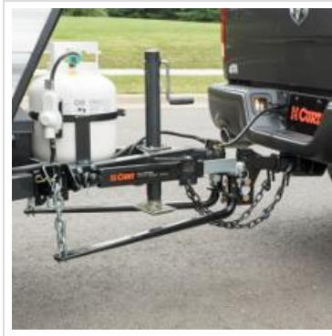
Image 6.5: A weight distribution hitch system connected, designed to improve towing stability and distribute load.
