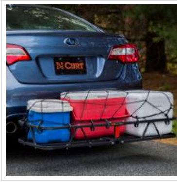
Image 6.4: A vehicle utilizing the hitch receiver for a cargo carrier, demonstrating its versatility beyond just trailer towing.
