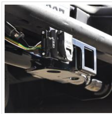
Image 6.3: The connection point for a trailer's electrical wiring harness, essential for trailer lighting and brakes.
