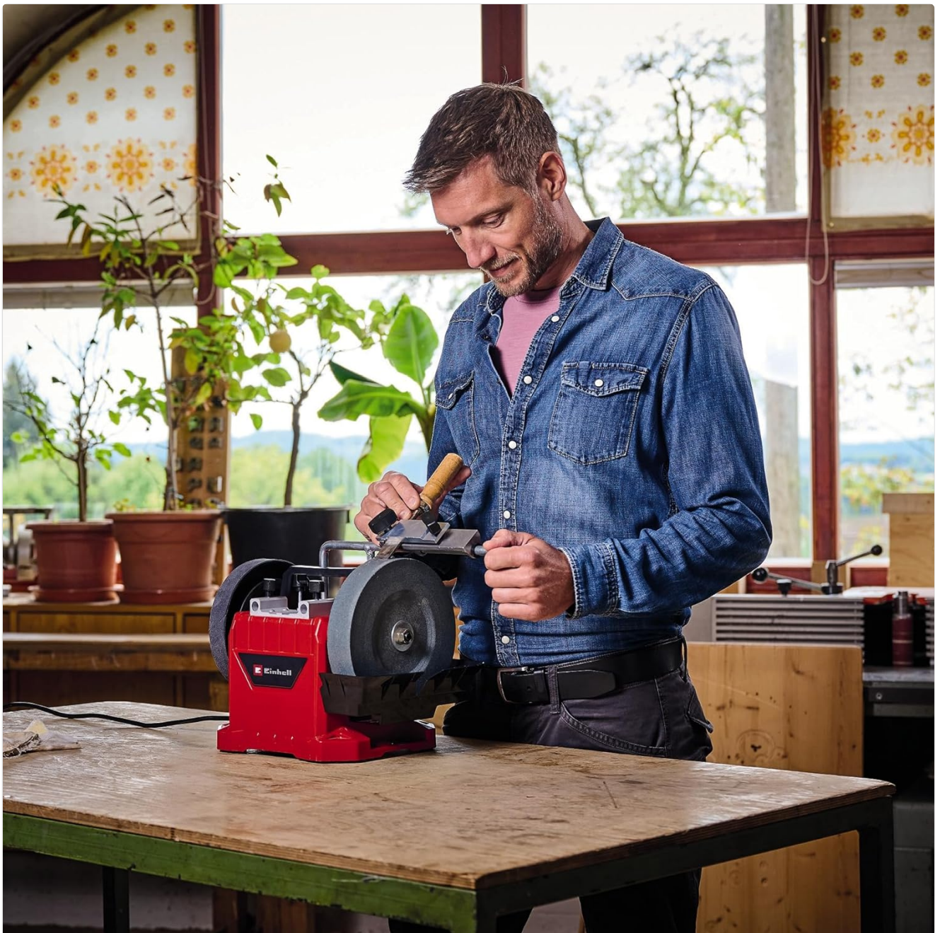
Figure 8: Proper technique for sharpening a tool on the wet bench grinder.
