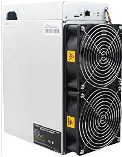
Figure 4.1: Front view of the Antminer Z15, showing the cooling fans.
