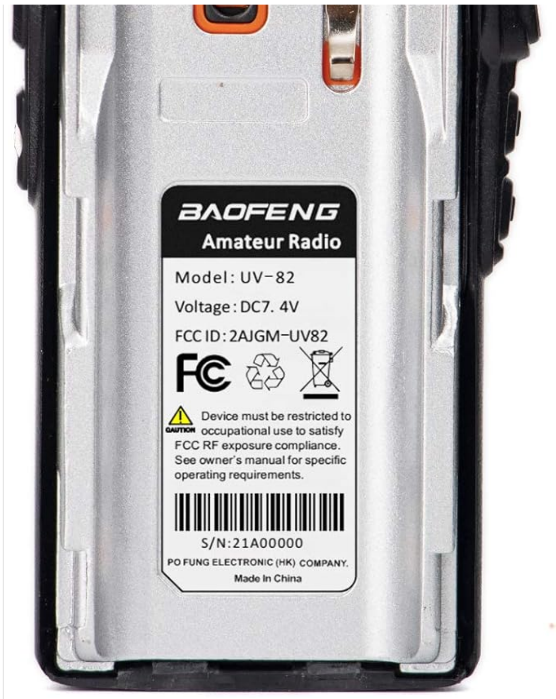
Figure 9: Back of the BAOFENG UV-82 radio, displaying the FCC ID and battery information.
