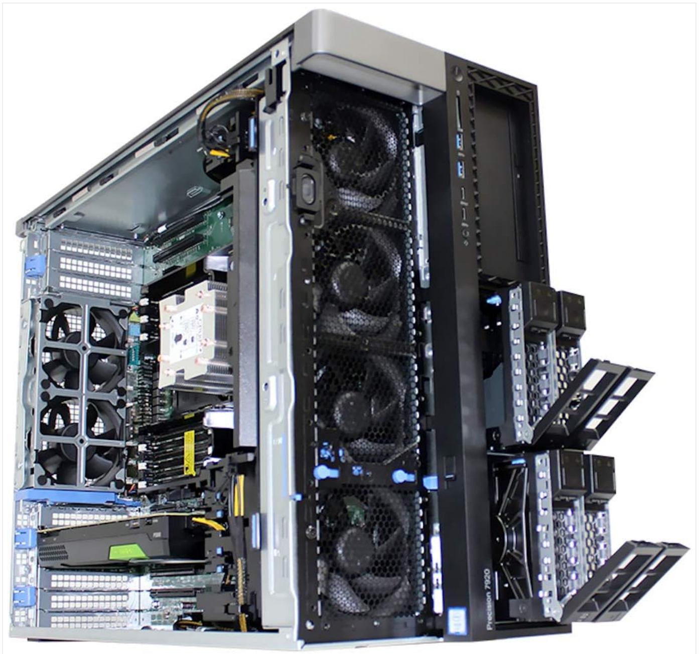
Figure 6: Internal view of the Dell Precision 7920 Tower Workstation with the side panel removed, showing the accessible drive bays and cooling system.
