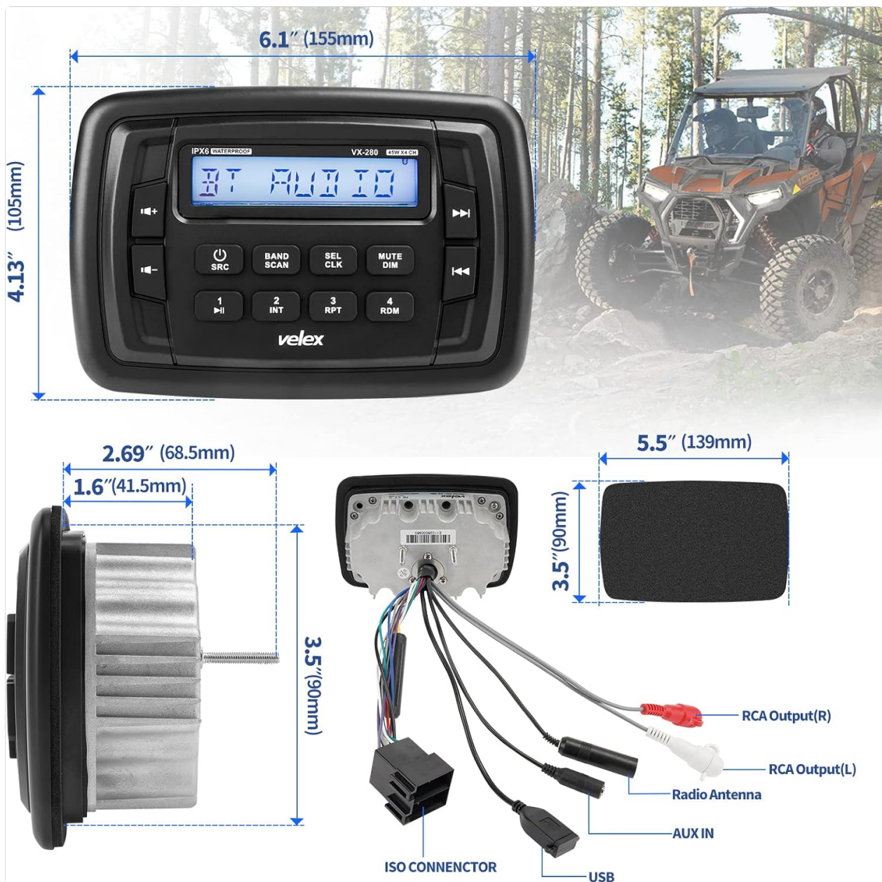
Image 4.1: Detailed dimensions and rear view of the Velex VX280 for mounting reference.
