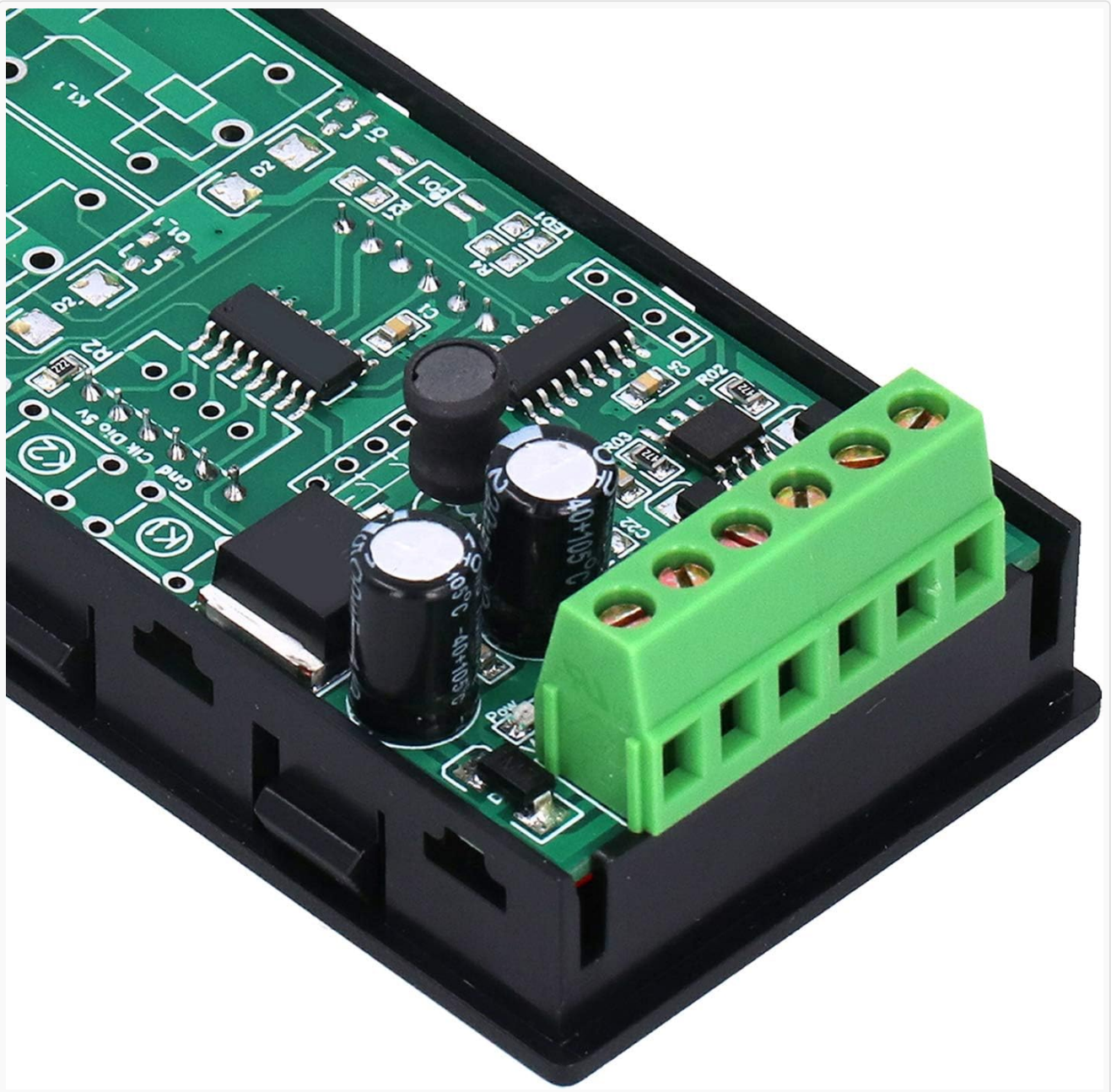
Figure 2: Close-up view of the terminal block, showing connection points for power and serial communication.
