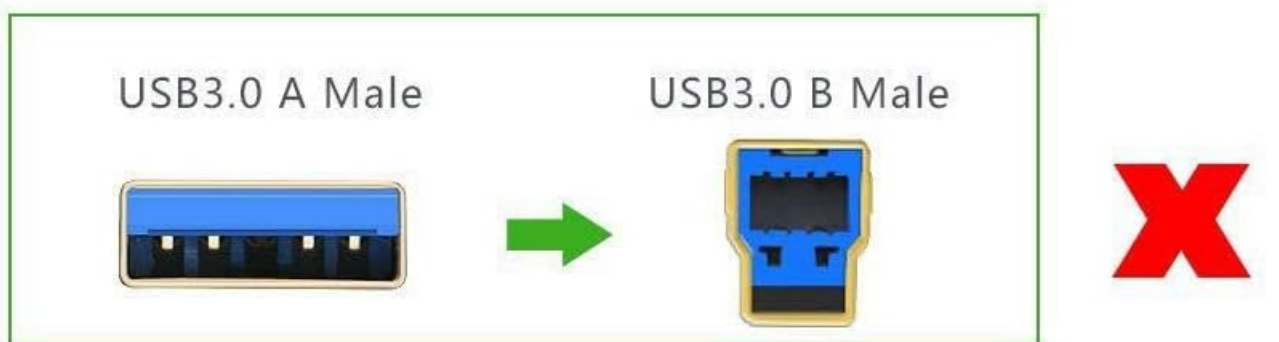
Figure 3.1: Comparison illustrating the difference between USB 2.0 Type A and B connectors (compatible with this cable) and USB 3.0 Type A and B connectors (not compatible).
