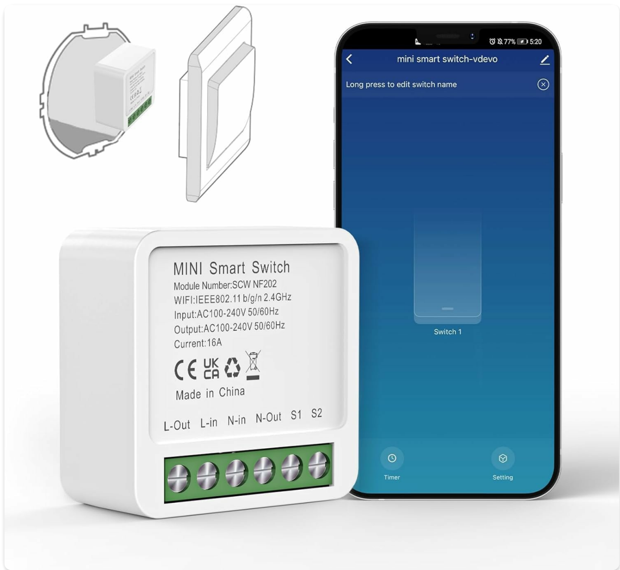
Image 1.1: Maxcio Mini WiFi Smart Switch with its mobile application interface. The switch is shown with its wiring terminals and compact design, alongside a smartphone displaying the 'Switch 1' control screen.
