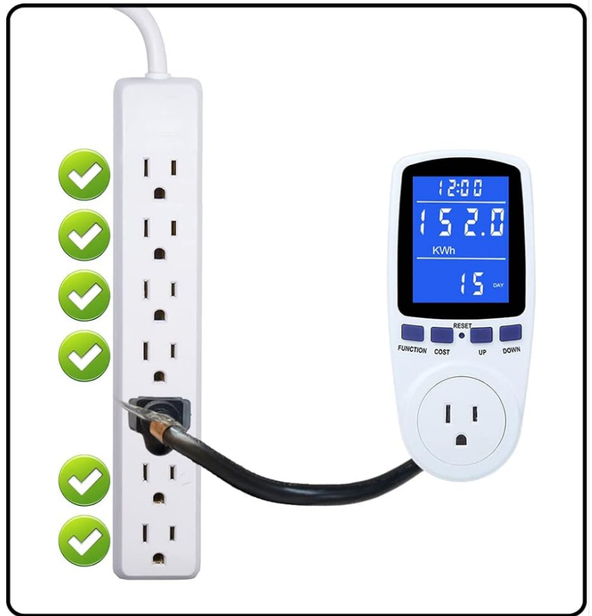
Figure 4.1: The power meter can be used directly or with an extension cord for convenience, preventing blockage of adjacent sockets.
