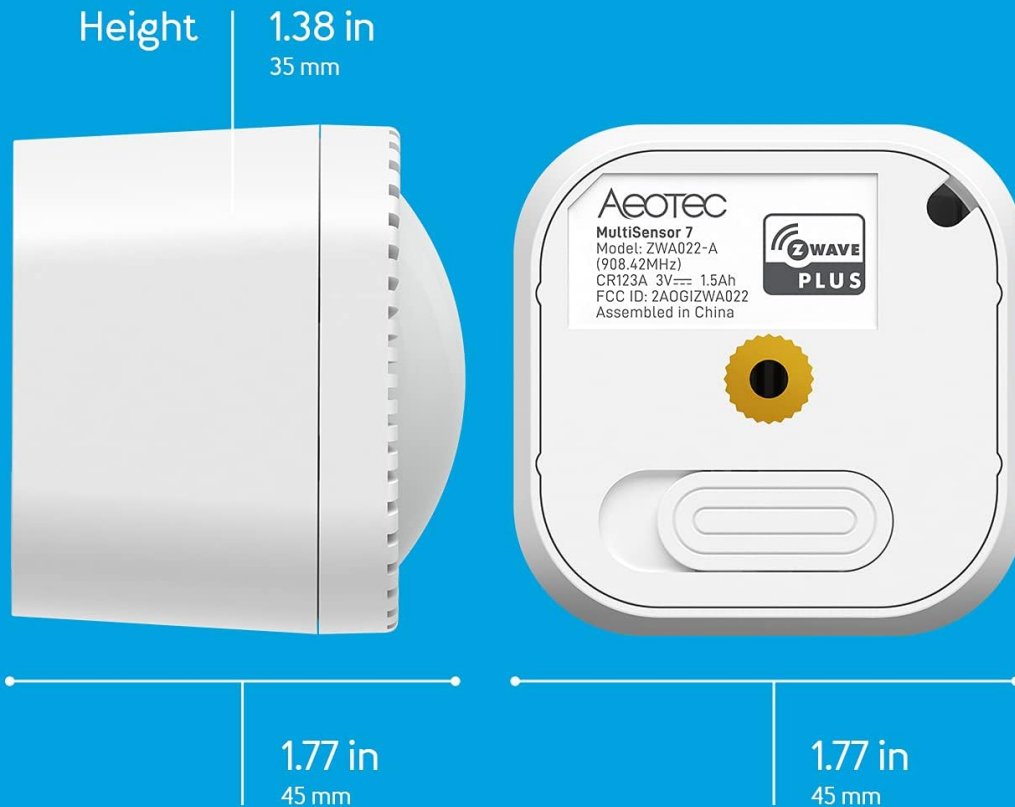
Image: Detailed dimensions of the MultiSensor 7.
