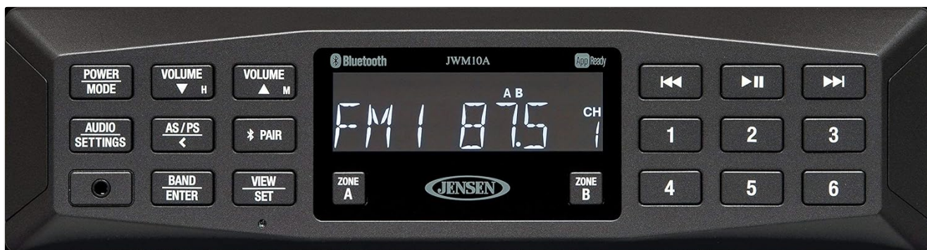
Image: Front panel of the Jensen JWM10A stereo, showing all buttons, the LCD display, and input ports.
