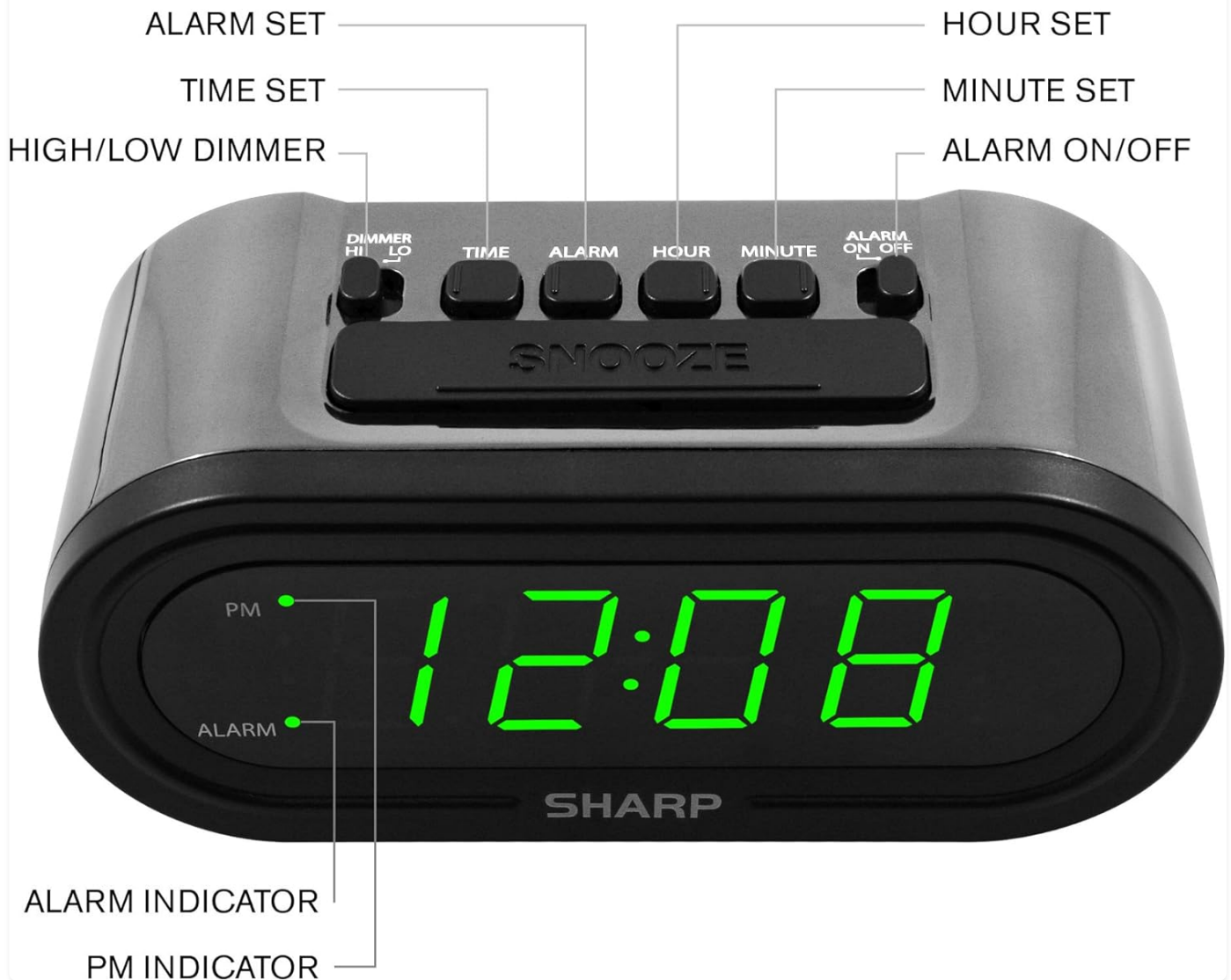
Figure 3: Top panel controls for setting time, alarm, and adjusting display.
